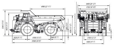
Overall dimensions are specified for basic configuration of the dump truck.
