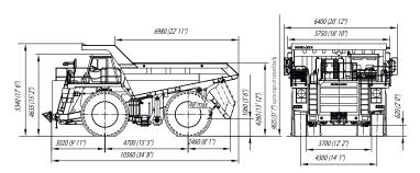
Overall dimensions are specified for basic configuration of the dump truck. The above specifications are subject to change without notice due to the continuous improvement of the vehicle design.
