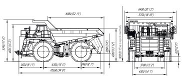
Overall dimensions are specified for basic configuration of the dump truck.
