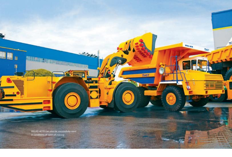
The loader has a strong articulated frame and bucket capacity of 7.2 cubic meters. The beam lifts a loaded bucket in 8.5 seconds, lowers it in 6 seconds and dumps it in 3.2 seconds.
