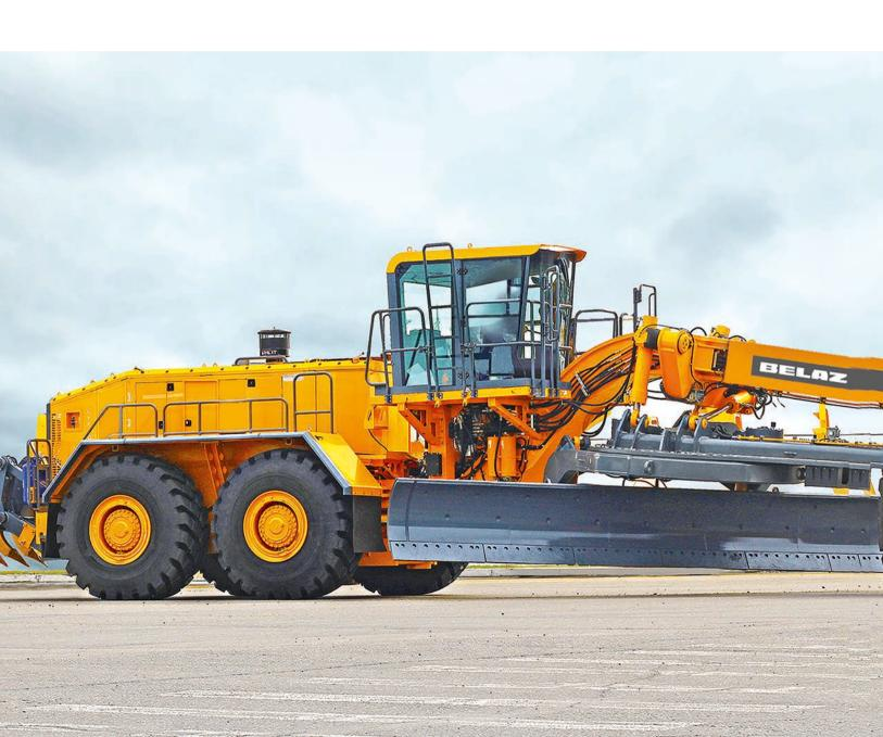
BELAZ Grader will lay and service technological roads, prepare convenient areas for reversal movements and parking vehicles, and also move large volumes of soil while planning and profiling working areas and slopes. Grader is also indispensable for clearing roads off snowdrifts. In general, this kind of mining equipment influences the safety of the road cuts.
