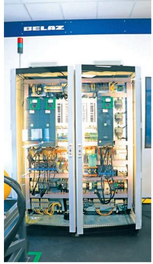
Load bench simulating the operation of internal combustion engine and motor-wheels  $% \left( {{{\rm{D}}_{\rm{B}}}} \right)$
