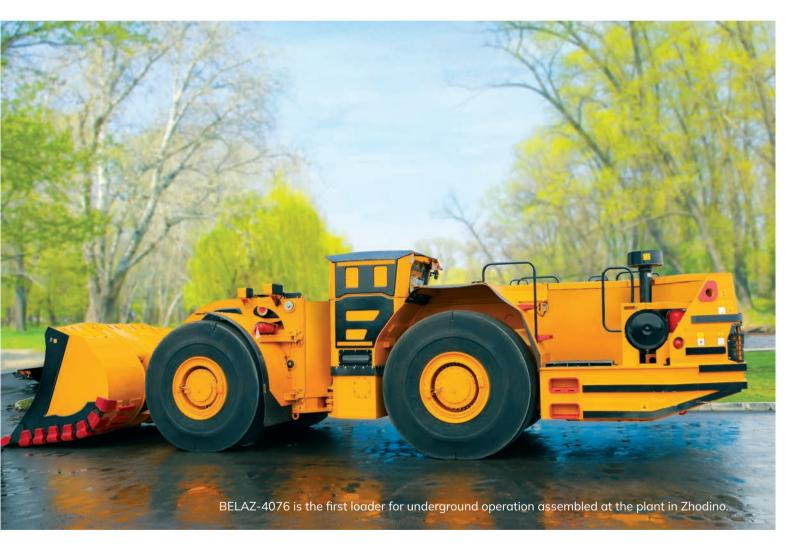
Developing the line of equipment for underground mining, BELAZ has created a new loader, model BELAZ-4076 with payload capacity of 17.2 tons.
