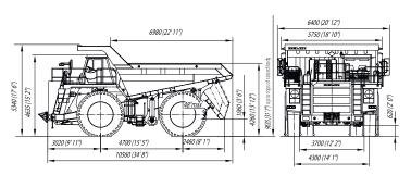
Overall dimensions are specified for basic configuration of the dump truck. The above specifications are subject to change without notice due to the continuous improvement of the vehicle design.
