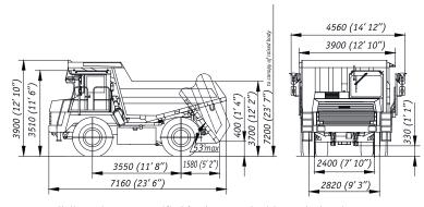
\*Overall dimensions are specified for dump truck with standard options
