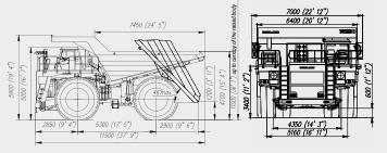
Overall dimensions are indicated for the basic configuration of the dump trucks.
