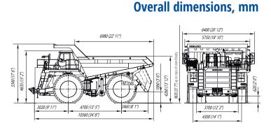
Overall dimensions are specified for basic configuration of the dump truck. The above specifications are subject to change without notice due to the continuous improvement of the vehicle design.
