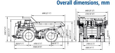
Overall dimensions are specified for basic configuration of the dump truck.
