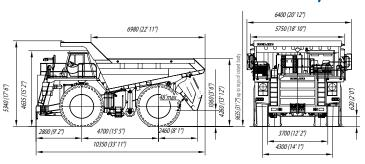
Overall dimensions are specified for basic configuration of the dump truck. The above specifications are subject to change without notice due to the continuous improvement of the vehicle design.
