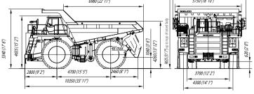
Overall dimensions are specified for basic configuration of the dump truck.
