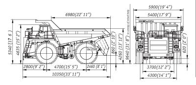
Overall dimensions are specified for dump truck with standard options
